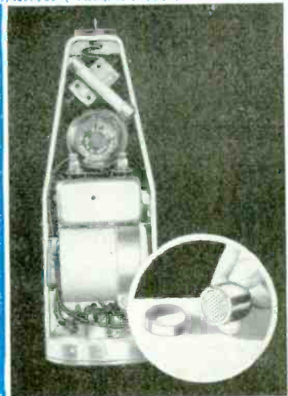
The amplifier is contained within the case of Western Electric's 640AA condenser mike. Mike (inset) screws on end.
