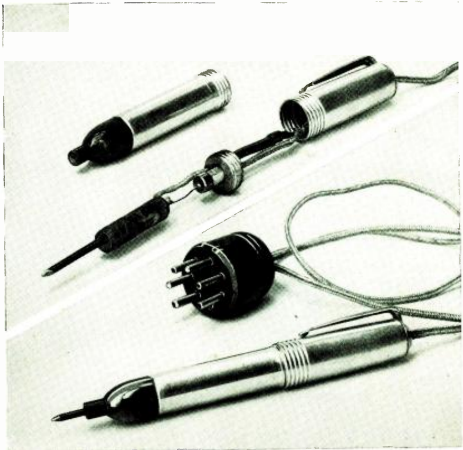
Fig. 6—Compact crystal probe for use with a v.t.v.m. is built in a small penlight case.
